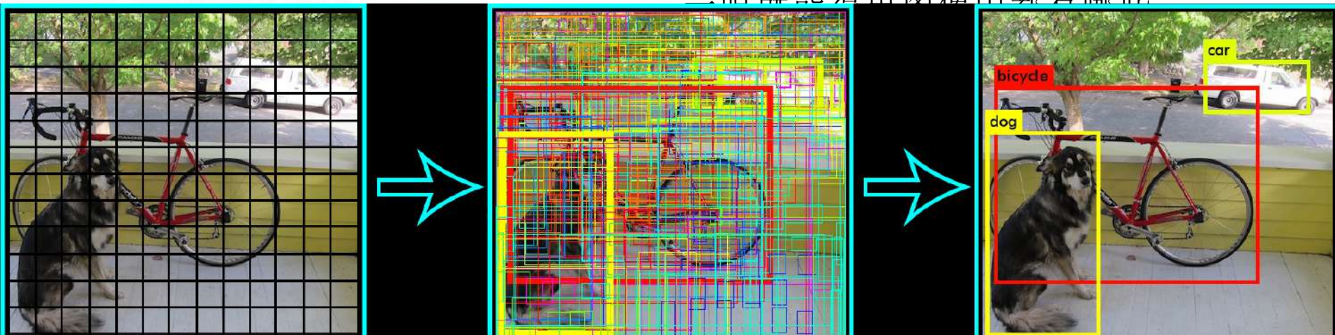
Figure 2: The Model. Our system models detection as a regression problem. It divides the image into an S \times S grid and for each grid cell predicts B bounding boxes, confidence for those boxes, and C class probabilities. These predictions are encoded as an S \times S \times (B * 5 + C) tensor.
