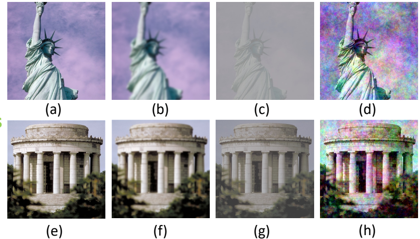
Demonstrations of the global distortions (a/e: reference image, b/f: Gaussian Blur, c/g: global contrast decrements, d/h: additive pink Gaussian noise)
