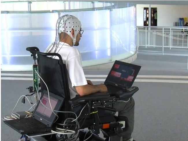
Control a wheelchair via EEG
